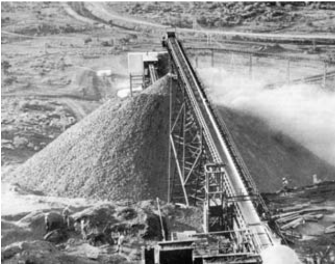
Primary stockpile of iron ore (hematite) at a mine run by RTZ in Australia, 650 miles NNE of Perth. When discovered, it was one of the world's largest deposits of high grade ore. (RTZ News, December 1966)
