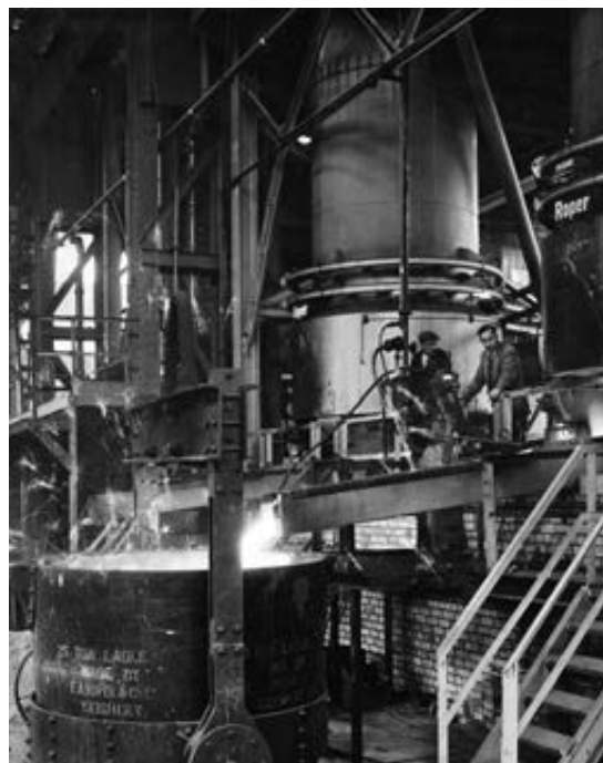
Consett Men of Steel: a hot and hazardous environment as molten steel runs into a 25 ton ladle, c1950s
